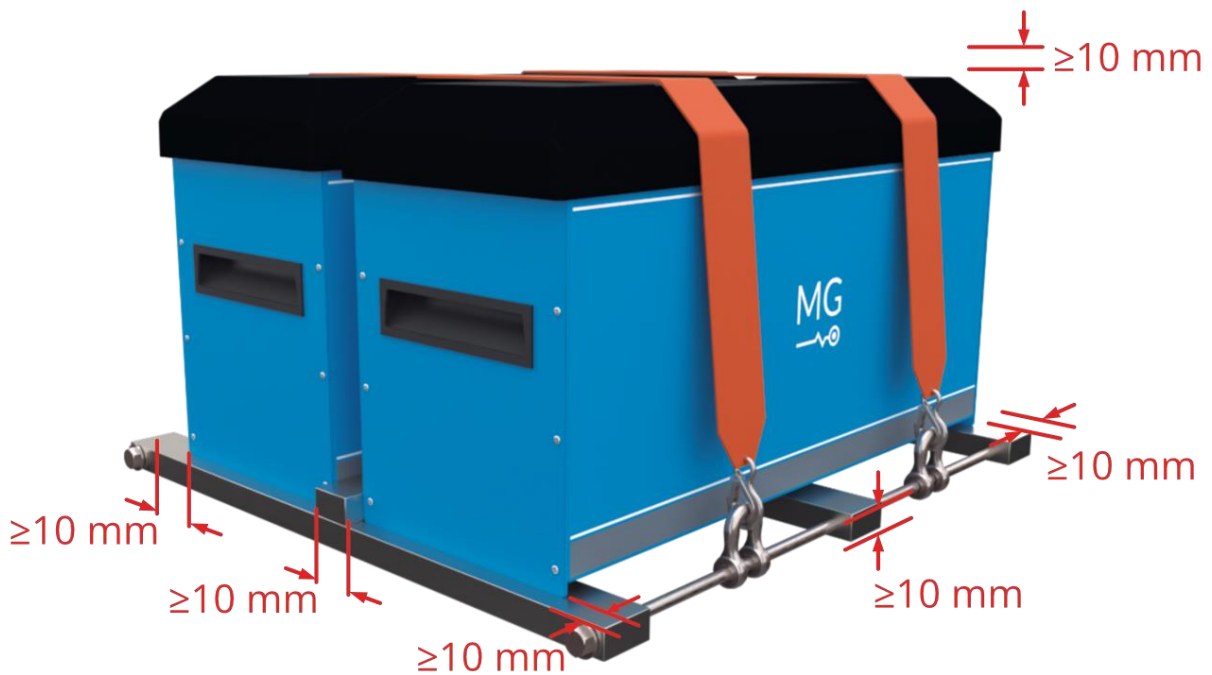
Figure 12 - Battery spacing requirements
